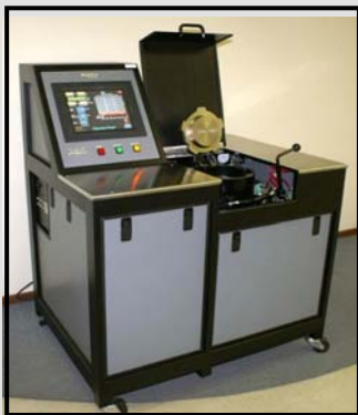
Fig. 2- Radiflo Mark VI Pressurization Unit
