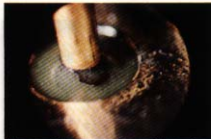
Figure 8, dye exiting through a thumbnail chip of a meniscus seal in a part with a 3 \times 10^{-7} atm. cc/sec. leak rate.
