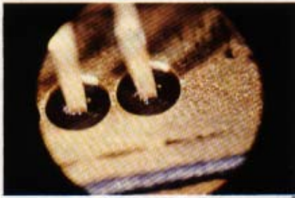
Figure 5, a hybrid with 5 \times 10^{-7} atm. cc/sec. leak rate in a brown glass header.
